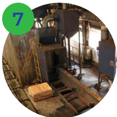
7 VỆ SINH - PHUN BÌ Shot blasting
